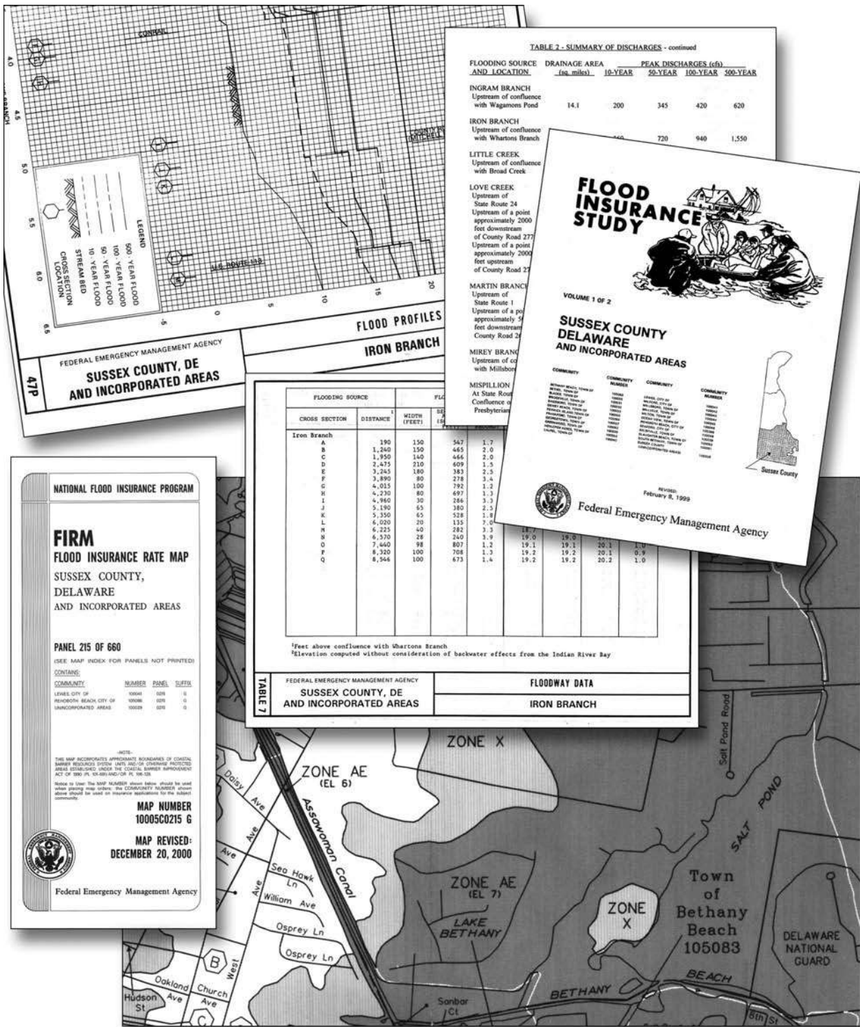
Figure 4-1. Portions of an FIS and a FIRM.
