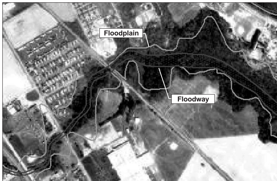
Figure C-6. Floodwaters in the floodway (dark gray) will have higher velocities than those in the flood fringes (between black and gray).
