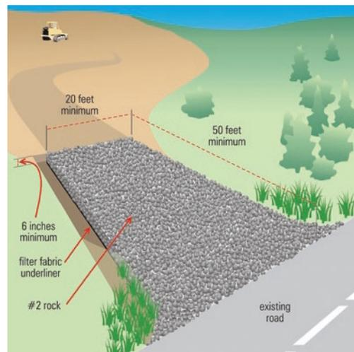
Figure 14. Illustration of a stabilized construction exit.
